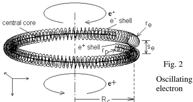
The physical dimensions of this structures are:  $R_C$  - Compton radius of electron (known),  $r_e$  -
