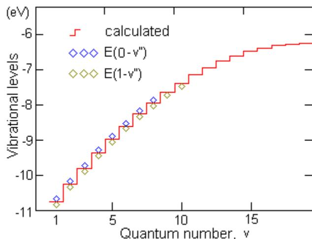
**Fig. [9.24].** Energy levels  $E_v$ , (eV) calculated by Eq. (9.23) and vibrational levels of the optical transitions  $E(0-v'')$  and  $E(1-v'')$ , corresponding to two QM spin values. The calculated levels are shown by step line, while the optical transitions by diamonds.
