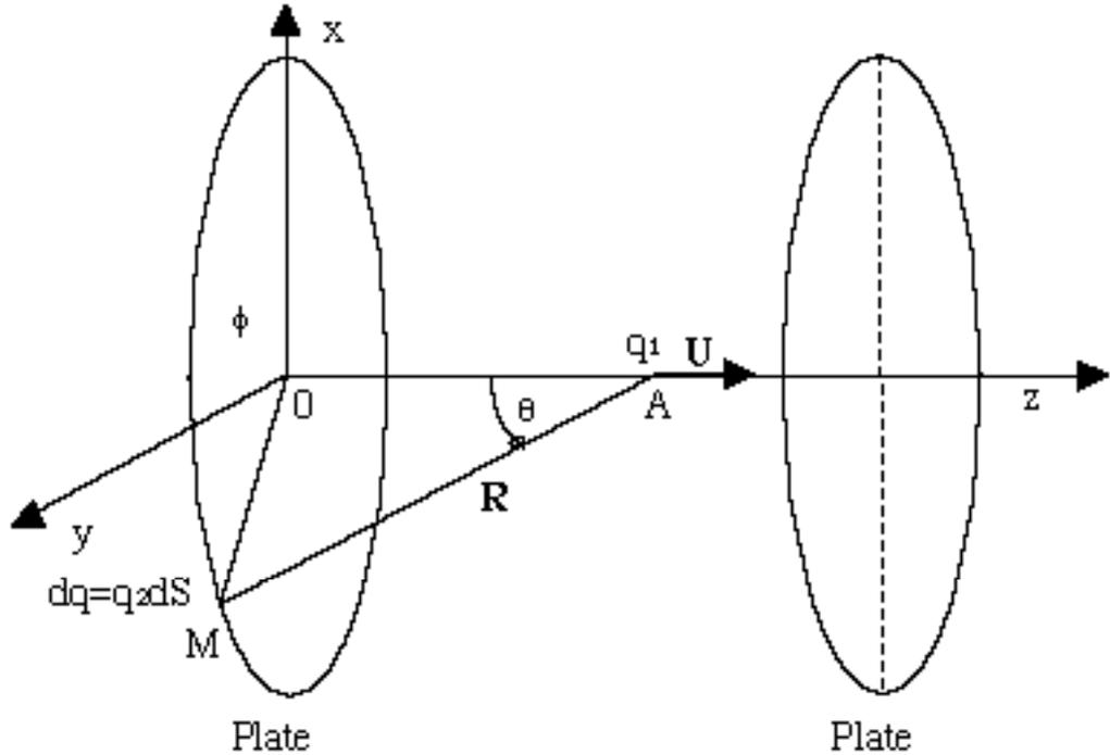
Figure 3 : charge  $q$  accelerated between the two plates of a capacitor
