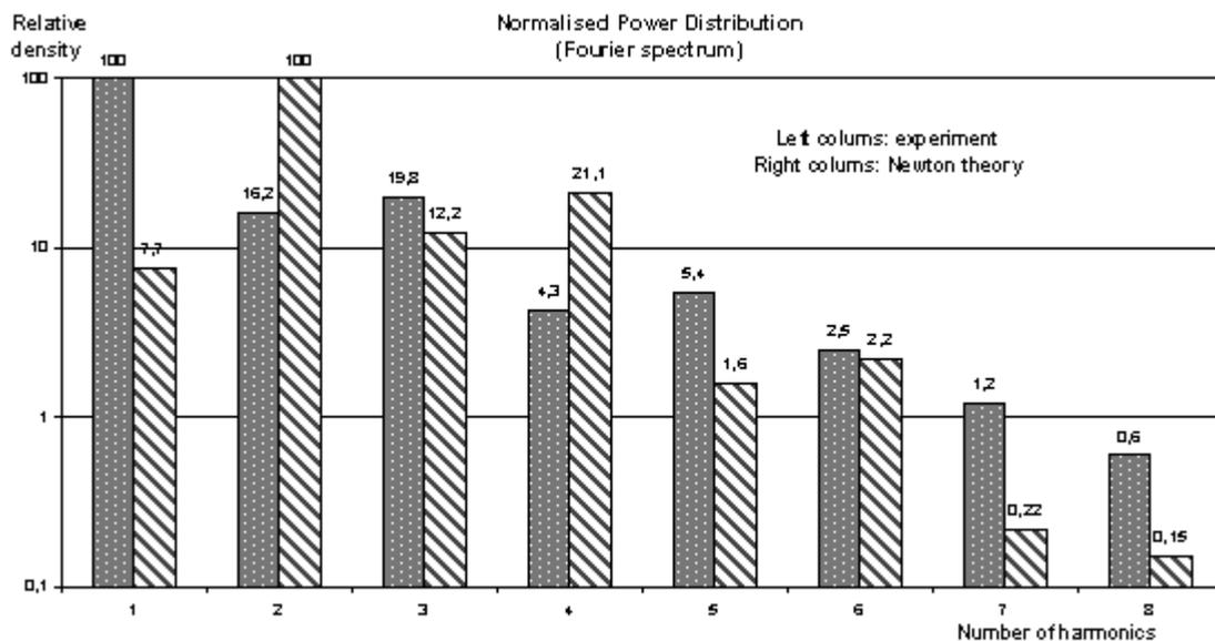
**Figure: 3. The Fourier spectrum of measured and calculated pendulum movement.**
