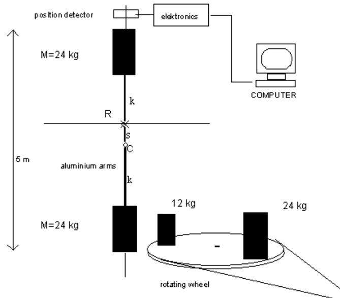
**Figure 1. The setup for the gravity measurement.**
